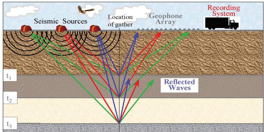
Figure 1. This diagram shows how the angular relationship varies from trace to trace in a common midpoint seismic gather. Each set of colored lines represents the ray paths of some of the energy contributing to an individual trace in the seismic gather. (All images courtesy of *e-Seis*)
